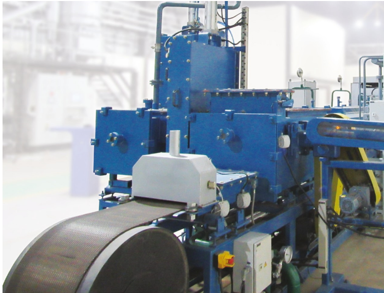
Fig. 3 Because parts enter and exit the furnace via a side entrance on the LGC, the front and rear openings through which the conveyor belt passes do not require the same headroom as in a typical mesh belt furnace
