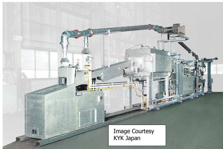
Fig. 7 The 'humpback' construction of inclined and extended front and rear tunnels in continuous brazing furnaces reduces gas consumption by half, but there are limits to the angle of inclination to prevent parts sliding down the furnace belt.
