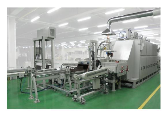
(-) 60°C dew point + <3 ppm O2 &  $\Delta T$  of 2.5°C within the furnace results in high quality sintered aluminium parts
