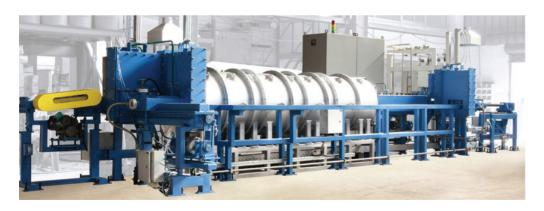
Nitrocarburising with nitriding potential (Kn) control
