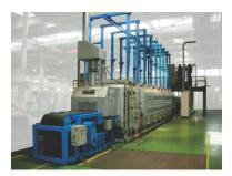
MESH BELT SINTERING TYPE RBO
