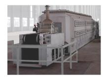
MESH BELT SINTERING TYPE EDB
