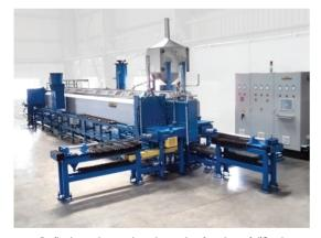
Boilerless steam treatment using humidified nitrogen; results in major energy savings and lower maintenance
