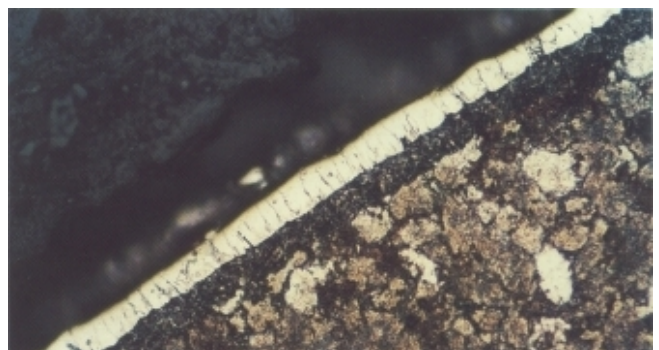
Ck 40. Austenitic Nitrocarburised @ 700°C and aged @ 350°C. Porous compound zone, backed by a Iron-Nitrogen bainite layer (Austenite Conversion).
