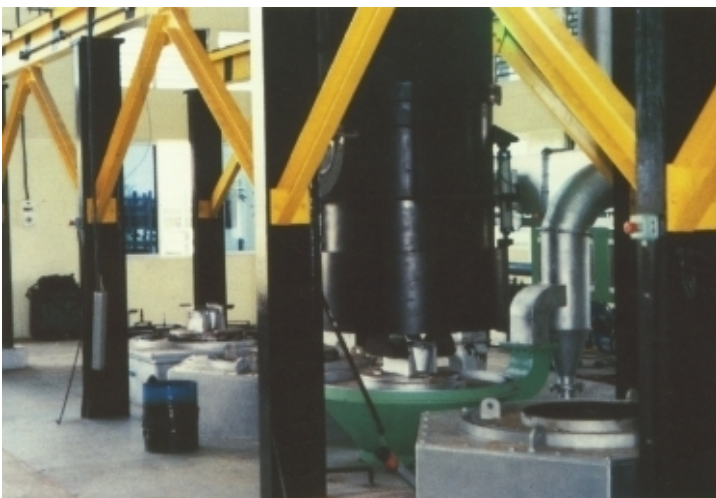
Partial view of a FLEXCELL comprising three hardening furnaces, two tempering furnaces, two quench tanks and one wash machine
