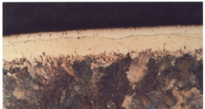
Ck45. Austenitic Nitrocarburised @ 650°C. Dense compound zone backed by an austenite layer and nitrogen diffusion zone.
