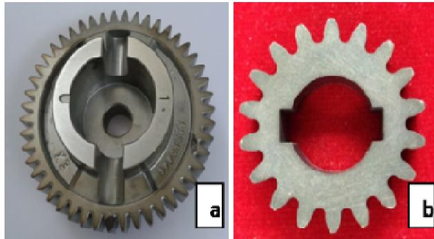
**Figure 2 Astalloy 85Mo components from Sintercom (a) and Hoganas (b)**
