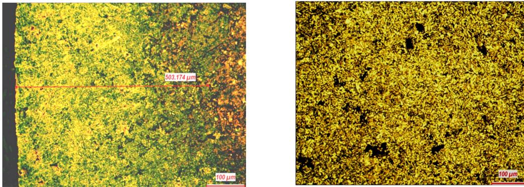
**Figure 6 Case (left) and core (right) microstructure (surface carbon potential 0.85-0.95%C)**
