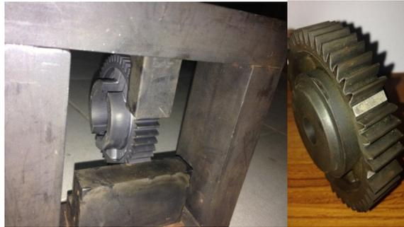
**Figure 9 Tooth strength test setup (left) and specimen after test (right)**
