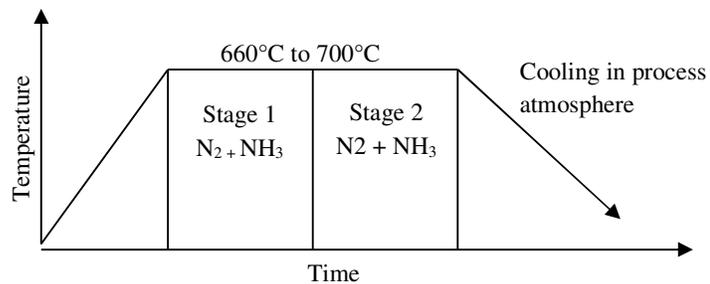
Fig.2 A typical POWNITE process cycle
