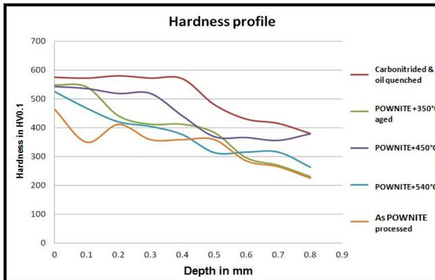
Fig. 10 Hardness profile from the surface of processed sprockets
