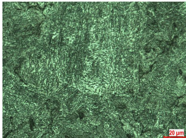
**Fig.8** Astalloy Mo + 0.6C Microstructure: Predominantly upper bainite with some ferrite and without any trace of martensite.
