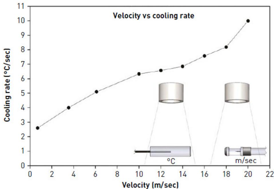
Fig. 6 Velocity vs cooling rate test. A  $\text{Ø}12.5 \text{ mm} \times 50 \text{ mm}$  Inconel rod with a  $\text{Ø}2.6 \text{ mm}$  N thermocouple inserted to the centre was heated to  $1080 \text{ °C}$  and subjected to a nitrogen stream from a D50 tube nozzle placed 120 mm above the rod
