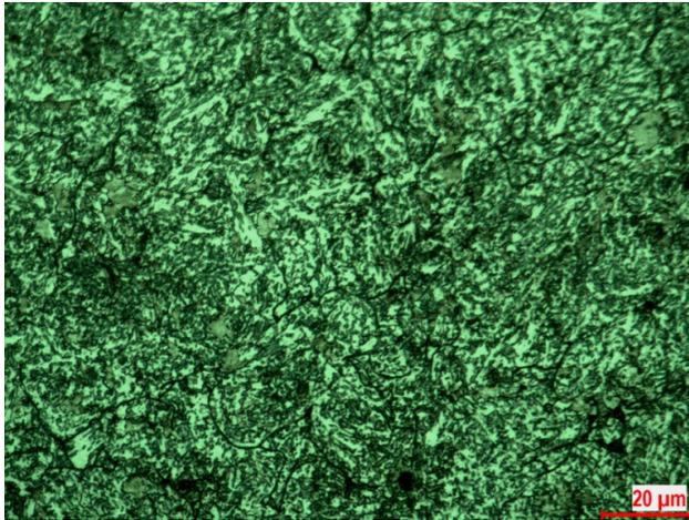
**Fig.6** Astalloy CRM Microstructure shows lower bainite with some ferrite and without any trace of martensite.
