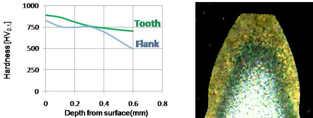
**Figure 3 Hardness profile and case structure of the improved case hardening trial, surface carbon potential of 0.85-0.95%C.**
