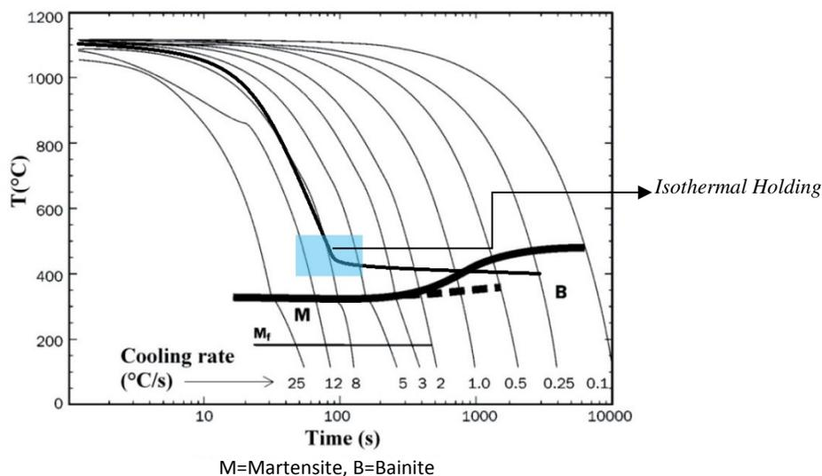
**Fig.1** CCT Diagram for Astaloy CRM
