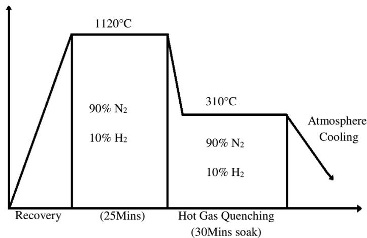
**Fig.4** Trial process cycle
