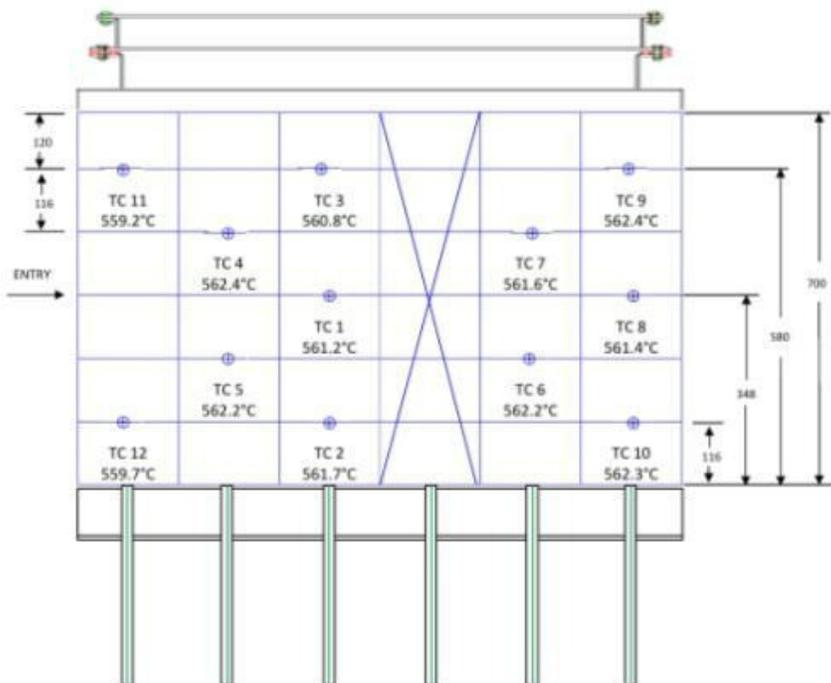
Fig. 7 TUS of the Al sintering furnace
