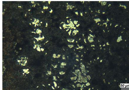
Fig. 9 Substrate microstructure - predominantly bainite
