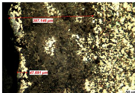
Fig.4 Surface structure showing a shallow layer of iron nitride with substrate of Bainite for N 9
