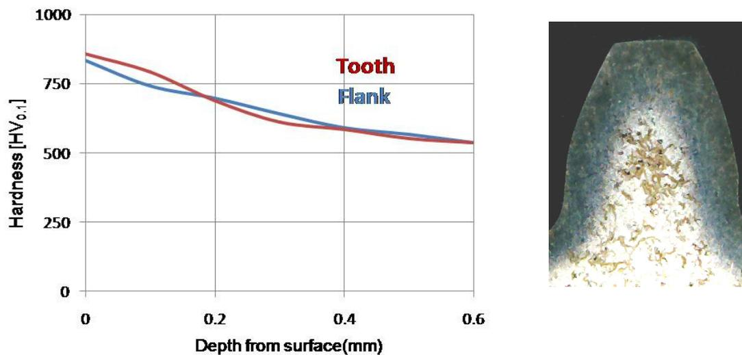
**Figure 5 Hardness profile and case structure of the trial in synthetic endogas atmosphere, surface carbon potential of 0.85-0.95%C.**
