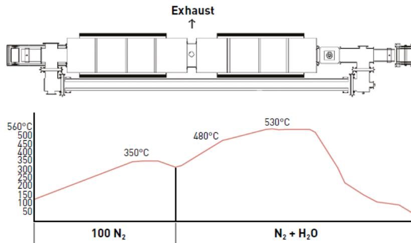
Fig. 8 An LGC furnace with features suitable for aluminium sintering and steam treatment would be suitable for the stress relaxation of soft magnetic alloy parts where required
