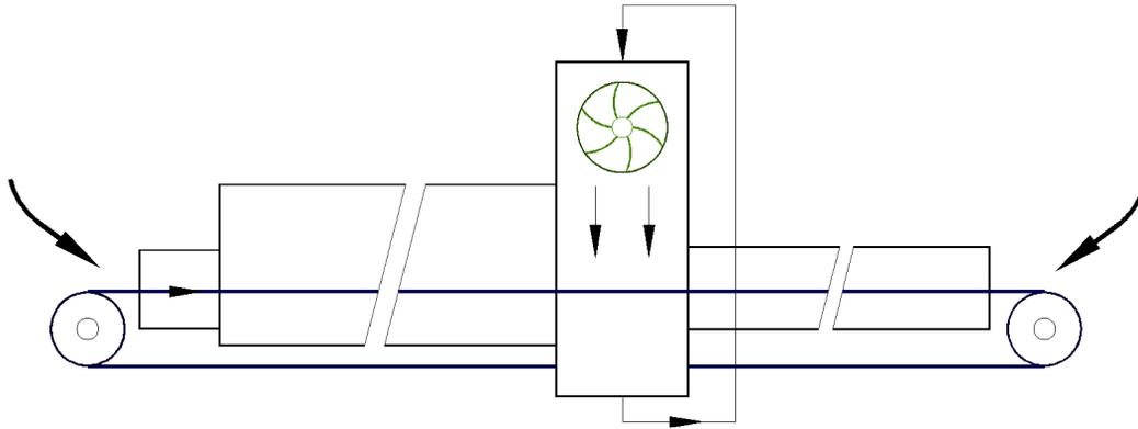
Fig. 5 When fan speed is increased to increase the cooling rate, air can often enter into the furnace tunnel, resulting in oxidation of sintered parts
