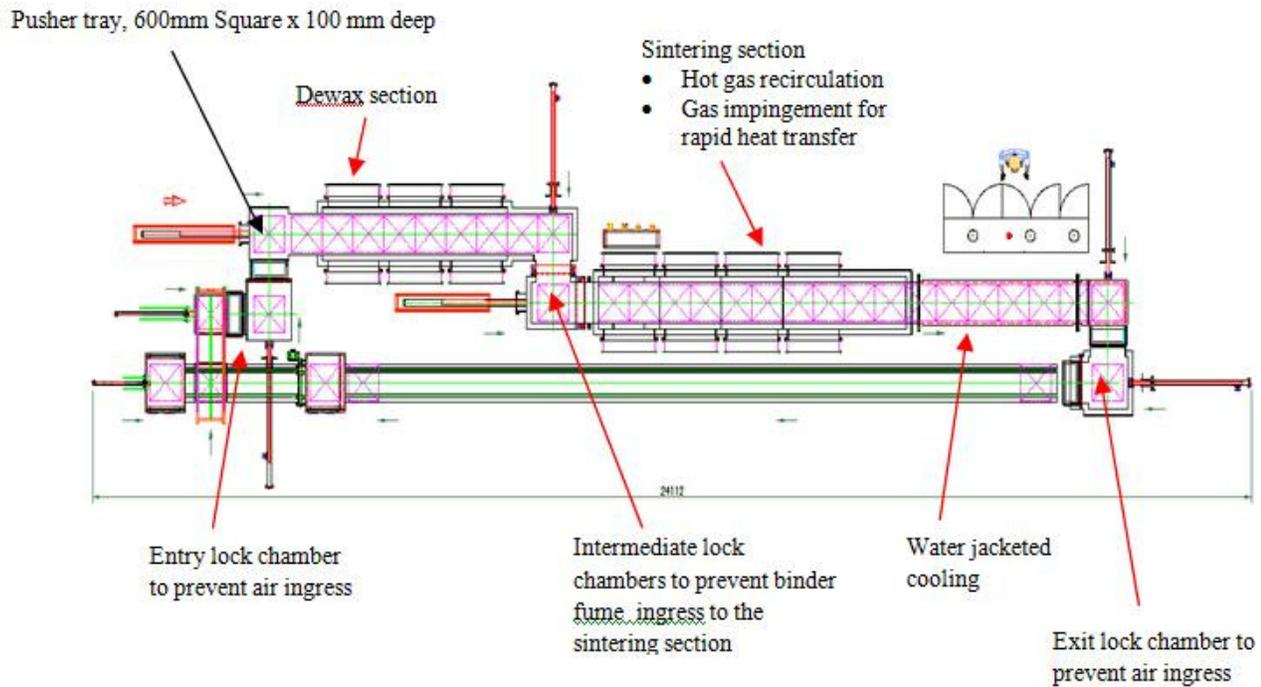
Fig.5 Furnace General Arrangement
