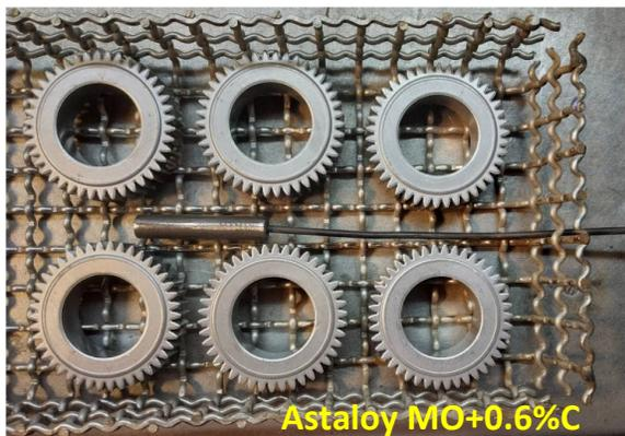
**Fig.3** Part loaded on a wire mesh tray with embedded trailing thermocouple
