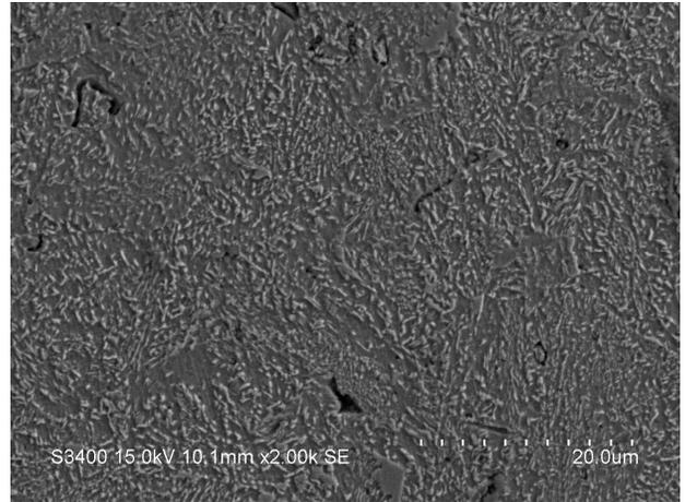
**Fig.7** Astalloy CRM SEM Micrograph shows predominantly bainitic structure.
