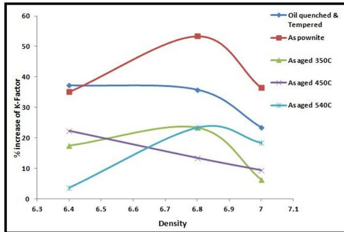
Fig. 12 % change as compared with sintered bush
