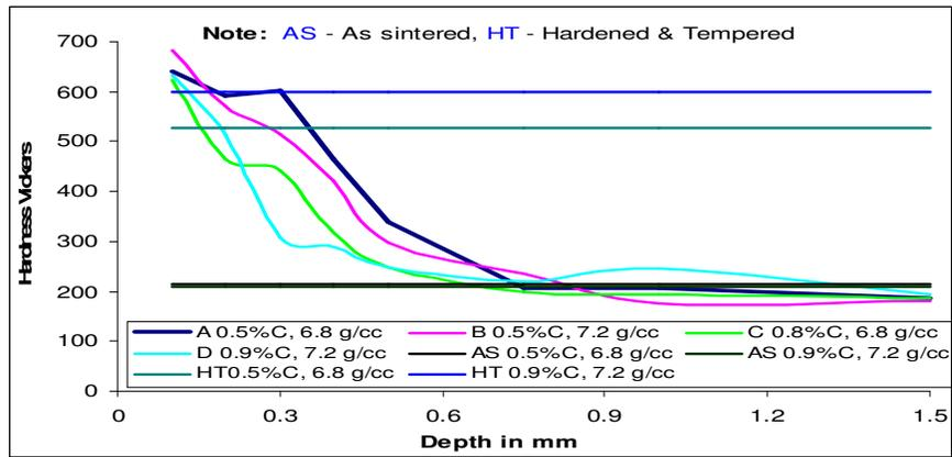
Fig. 6 – Hardness profile of Experiment N9
