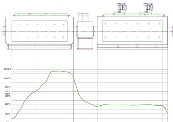
**Fig.2** Sinter (Bainite) Hardening furnace with Thermal Profile
