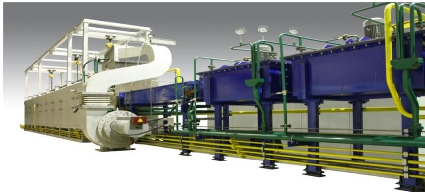
Figure 1: A typical continuous sintering furnace with gas quenching module
