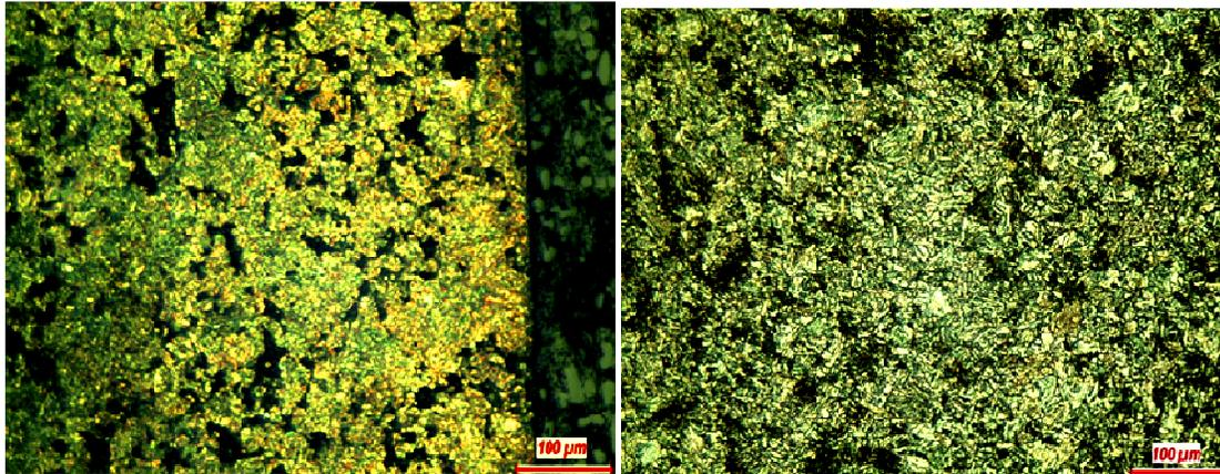
**Figure 4 Tooth flank (left) and core (right) microstructure, (surface carbon potential 0.85-0.95%C)**
