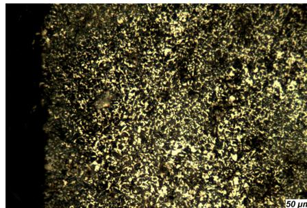
Fig.3 Surface structure showing Bainite with ferrite and without Iron Nitrides for N 5
