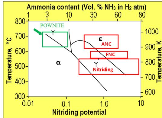
Fig. 1 The POWNITE process position in the Lehrer diagram
