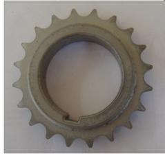
Fig 8 Material: C 0.5c, Cu 2.5%, Bal Fe
